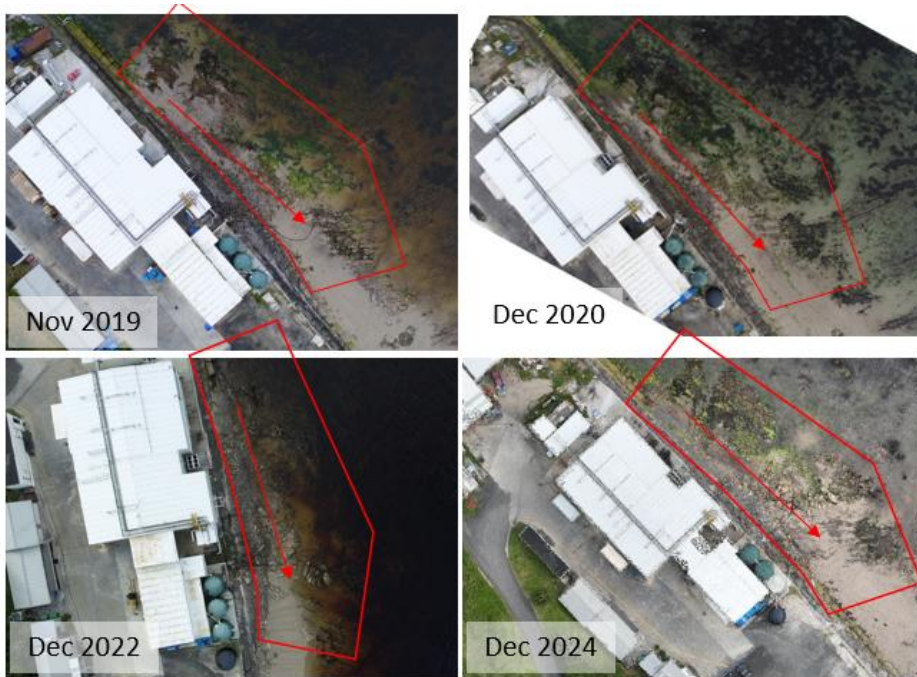
Figure 3.5: UAV photo analysis showing differences in Town Beach sand levels in front of the fish factory between Nov 2019 (top left), Dec 2020 (top right), Dec 2022 (bottom left), and Dec 2024 (bottom right). Arrow shows general easterly movement of sand
