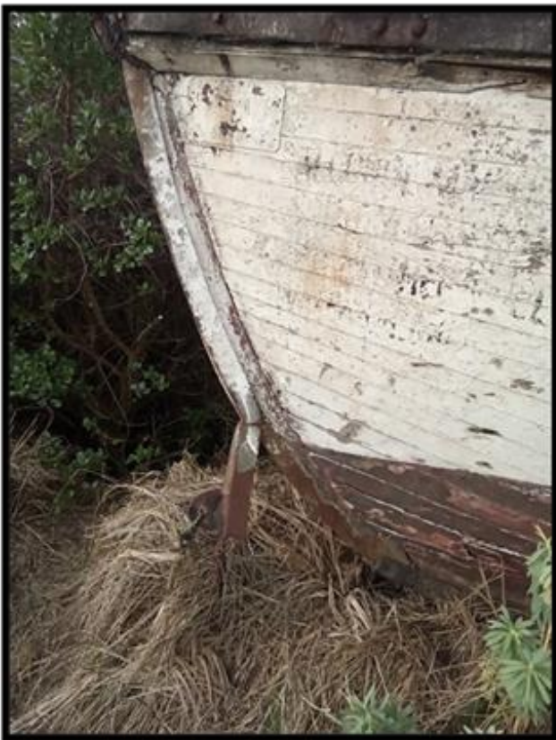
Figure 10 Bent stem capping
