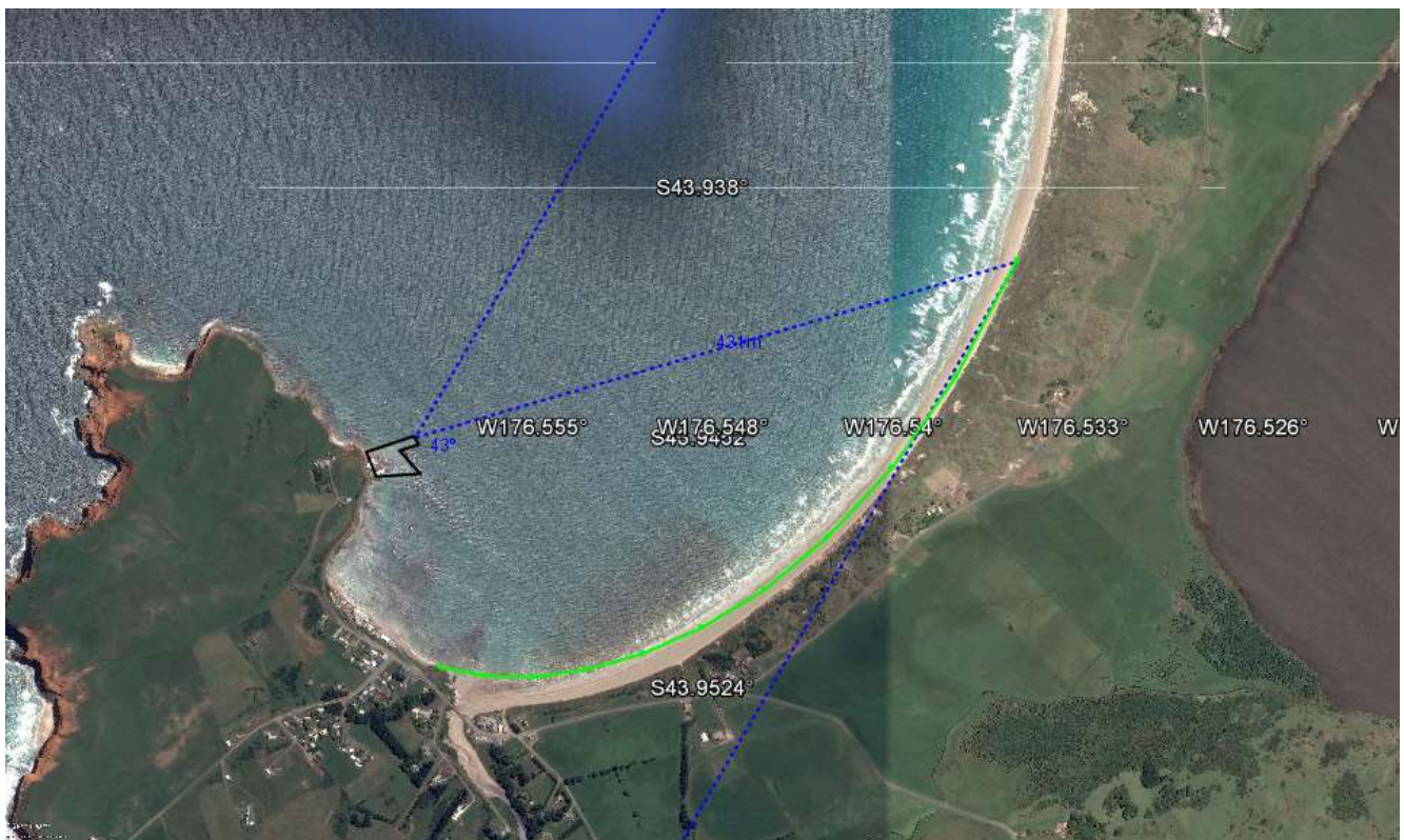
Figure 4-9 Analysis of an equilibrium planform for southern Waitangi Bay with reclamation and 60 m breakwater
