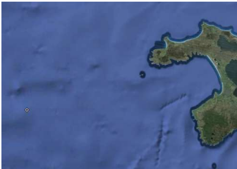
Figure 3 Proposed location of numerical wave output point offshore of Waitangi Bay
