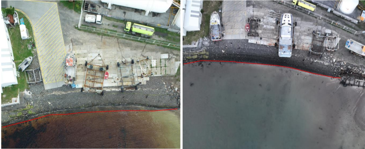
Figure 3.4: UAV images at photo-point monitoring at point Nov 2022 (left) and Nov 2024 (right). Red line shows gravel/sand interface.
