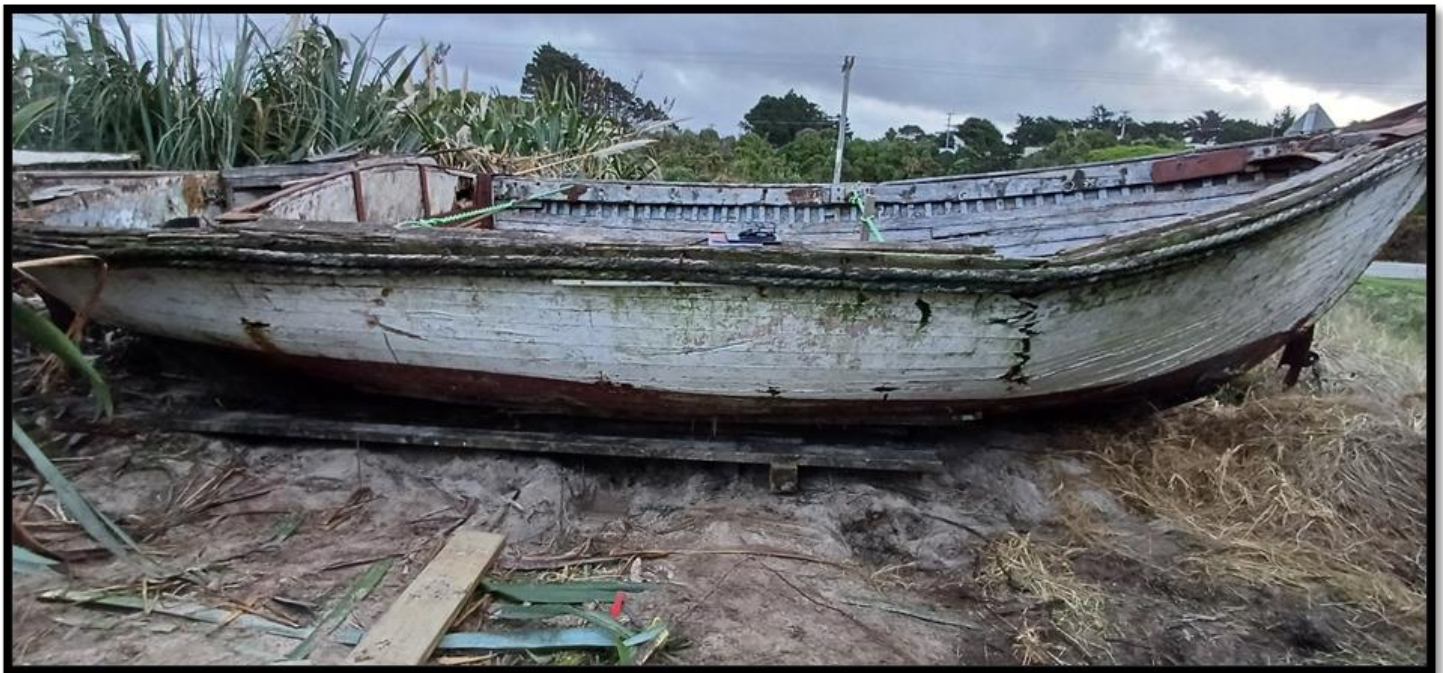
Figure 8 Starboard side planking. Note cracking
