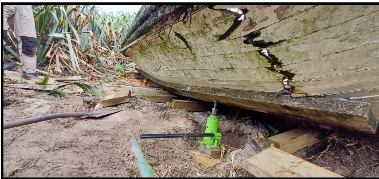
Figure 6 Surfboat getting lifted for inspection during survey.
