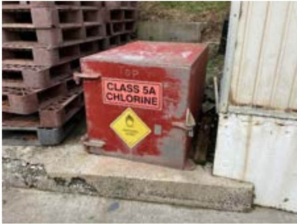
Fig. 7: Powdered chlorine stored next to truck washdown area.
