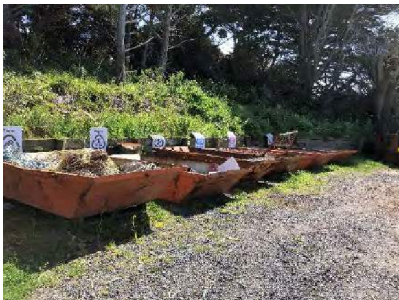
Figure B1-3: 3m³ gantry bins for diverse materials including rope nets.
