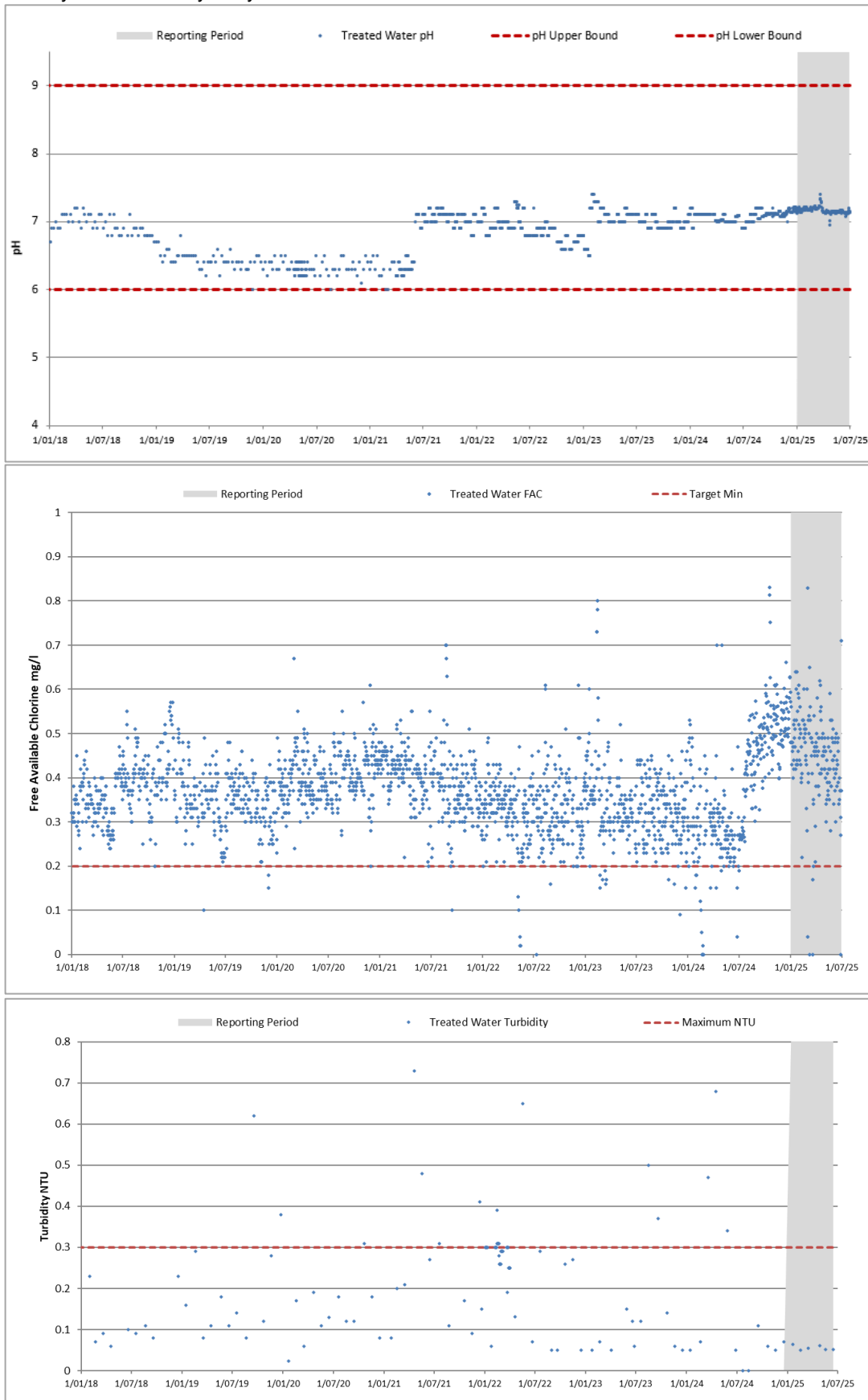
Figure 4: Waitangi treated water pH, FAC and turbidity
