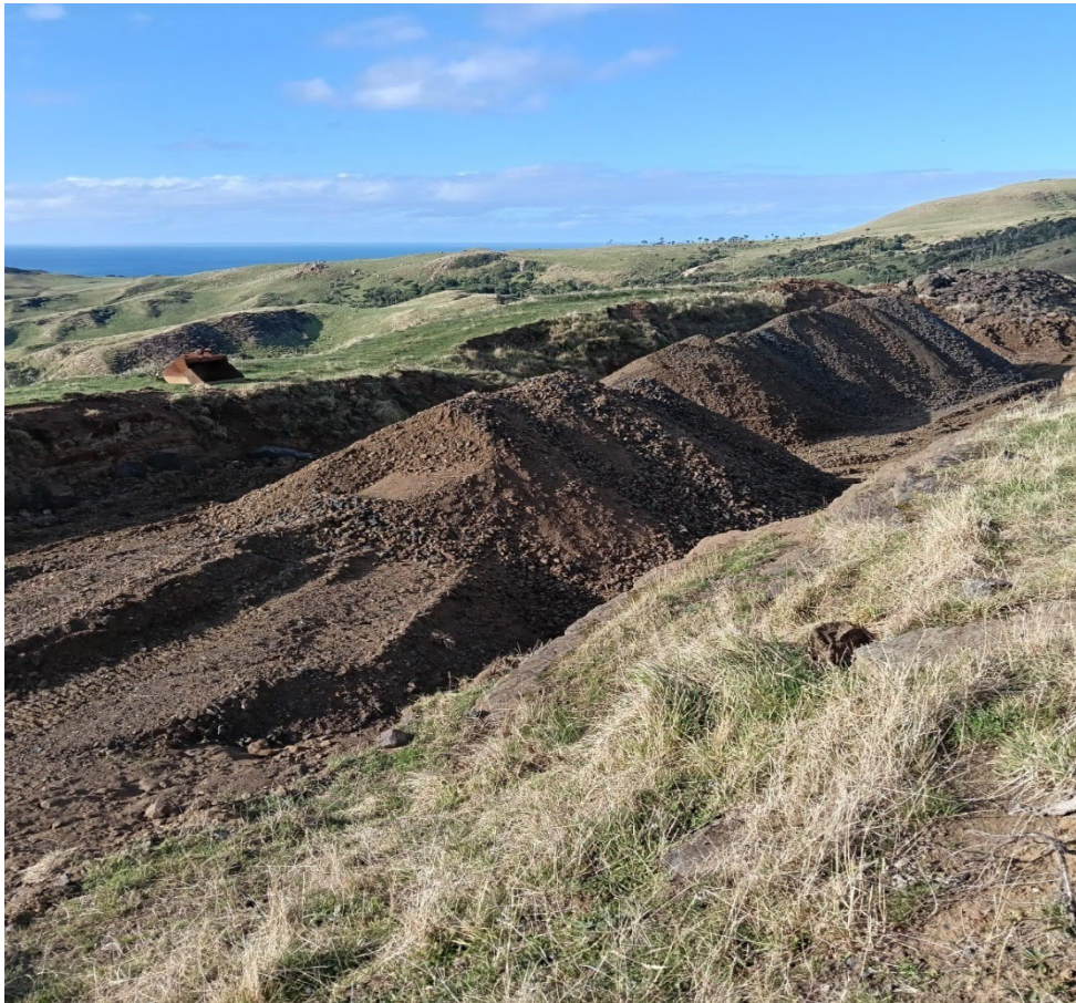
Crushed Metal For Roads On Pitt In Paddy's Pit
