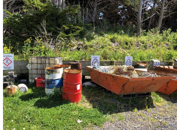
Figure B1-2: IBC used for storage of waste oil, with 3m 3 gantry bins.
