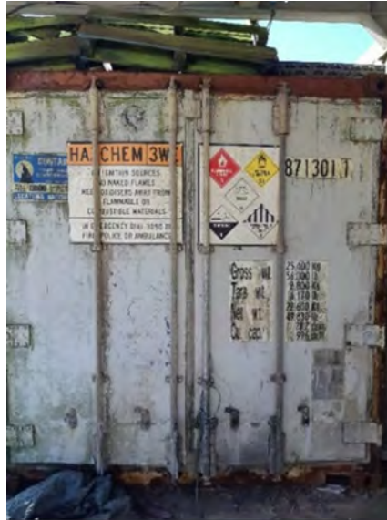
Fig 7. Label shows oxidisers and flammables stored in of Chlorine same container
