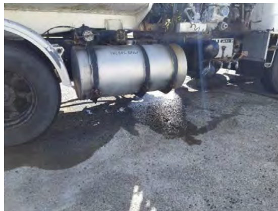
Fig. 31 Fuel tanker leaking fuel.
