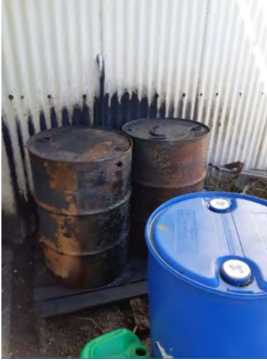
Fig 28. Old, leaking fuel storage barrels.
