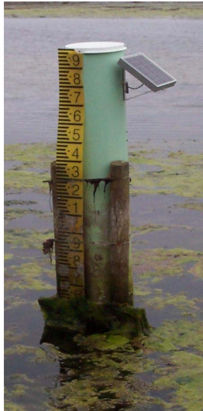
Figure 2a. Typical installation (the Mouth recorder) showing PVC tower supported by fence posts driven into the bed, with solar panel and staff gauge.
